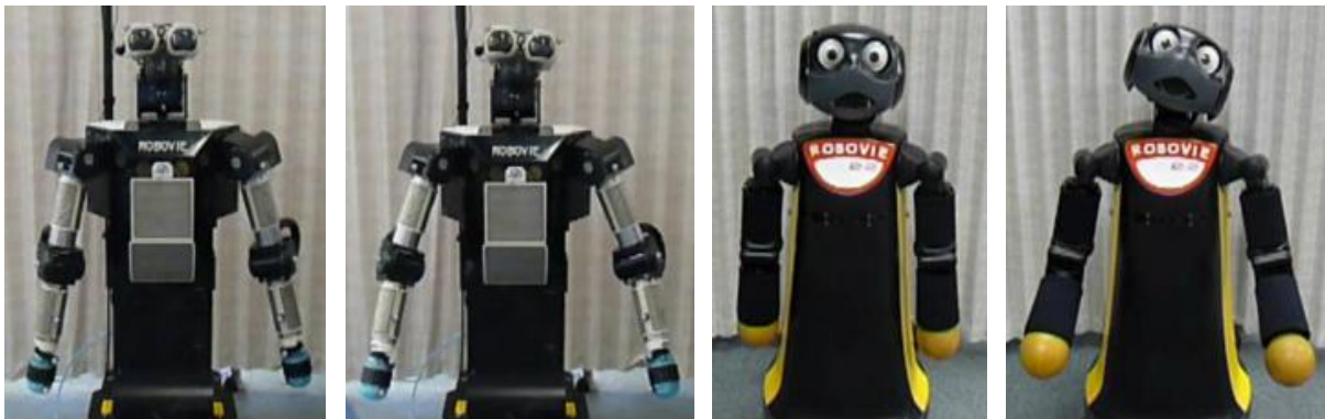
Figure 1: Robovie-II with its initial posture and during laughter (left, second from left); Robovie-R2 with its initial posture and during laughter (third from left, right)
