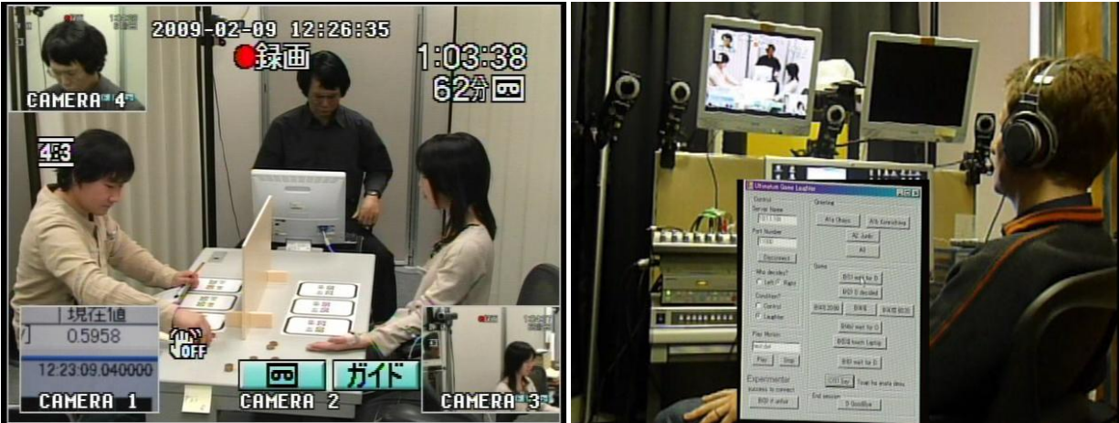
Figure 7: The combined view of all four cameras (left), which is used at the tele-operation console (right) to control Geminoid HI-1 remotely by means of buttons, which trigger predefined movements with utterances in Geminoid.
